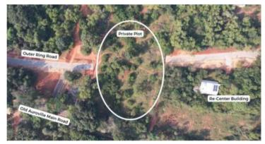
In Aurodam, the radial was partially built on Poromboke land and now ends abruptly. It was also built two meters too wide in one place, and at the wrong elevation meaning that it will not connect to the Crown as it is supposed to.
