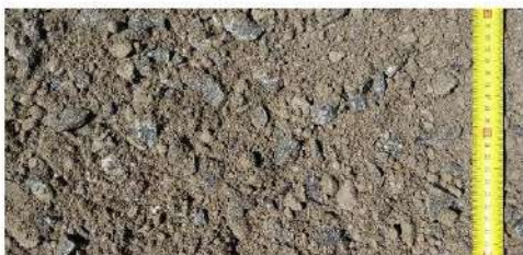
Fig. 69: Too many fines in the aggregate
