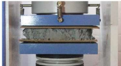
Fig. 50: Testing new pavers by Sri Annai Tiles
